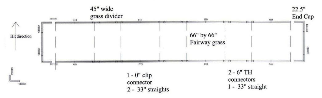
Frame parts required: 0" clips - 8; 6" TurfHound clips - 20: Corners - 4; 33" straights - 24
