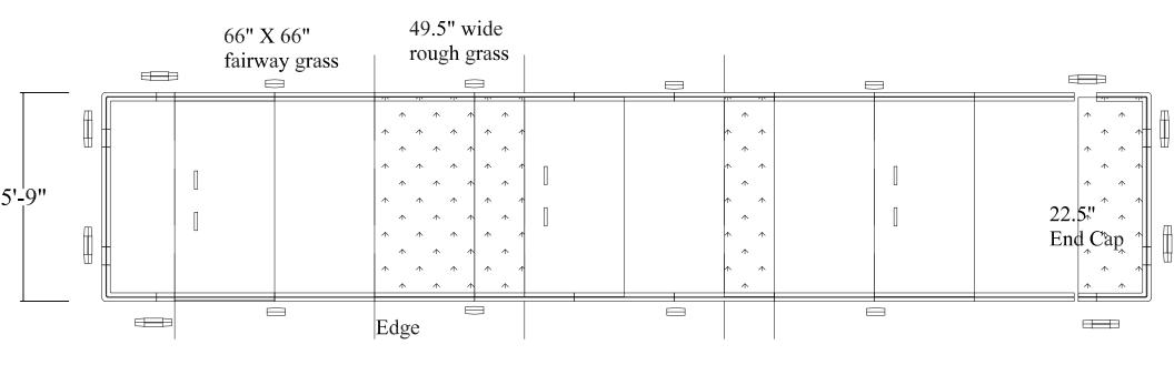
Frame end cap assembly; 0 - 0" quick connects = 1 - 33" straights = 4 - 6" quick connects = 1 - Right hand corner 1 - Left hand corner Turf End Cap Assembly; 1 - 22.5" x 66" end caps
