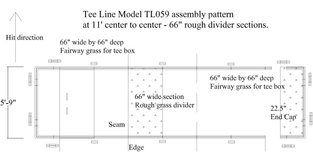
Frame end cap assembly; 0 - 0" quick connects = 1 - 33" straights = 4 - 6" quick connects = 1 - Right hand corner = 1 - Left hand corner Turf End Cap Assembly; 1 - 22.5" x 66" end caps
