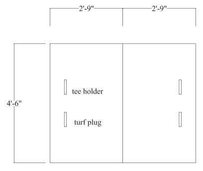
Two 33" by 54" turf pads fit inside the connected frame
